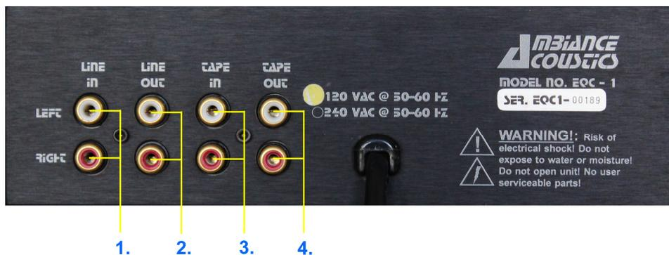
1. INPUT SOURCE (unbalanced): Mixing board, pre-amp out, or pre-out from a receiver or integrated amplifier (line level source) plugs in here
